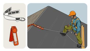
Left: A synthetic webbed anchor strap and a metal roof anchor (ridge anchor). Right: Fall-restraint systems prevent workers from falling from a work position or from travelling to an unguarded edge.
