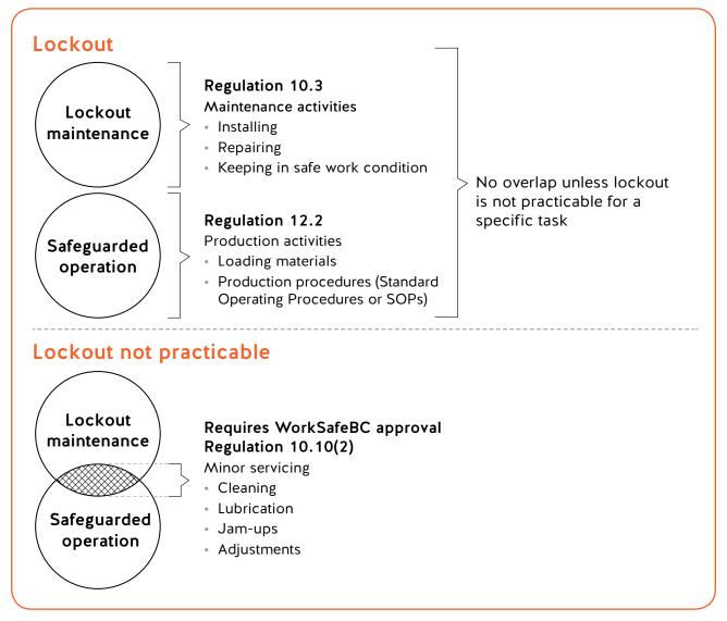
Figure 4: How safeguarding and lockout co-exist.
