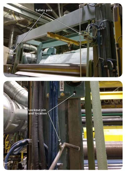
Figure 19: Pins used for safeguarding and lockout. (A) Safety pins that are part of a machine's safeguarding system for normal operating activities. (B) Lockout pin to be used during maintenance.
