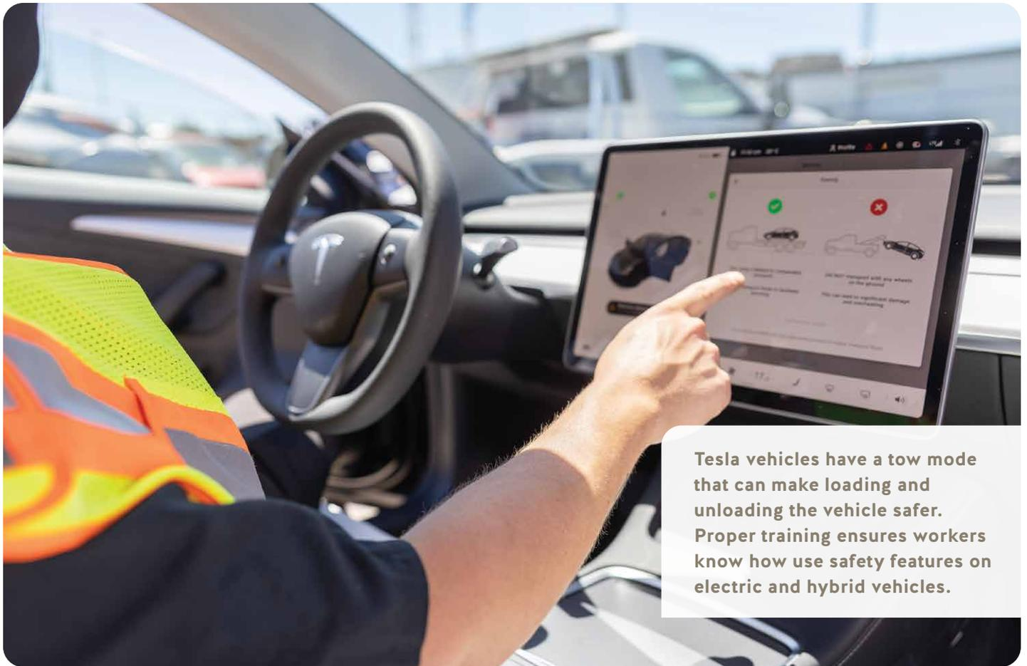
**Tesla vehicles have a tow mode that can make loading and unloading the vehicle safer. Proper training ensures workers know how use safety features on electric and hybrid vehicles.**
