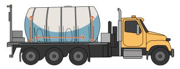
The arrows indicate how the weight of a live load and its centre of gravity can shift. Liquid sloshing around in the tank can have a significant effect on the vehicle's handling and stability.
