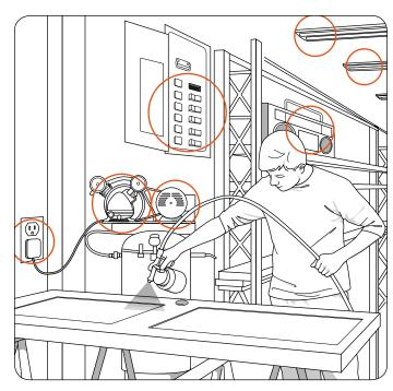
The drawing above shows some potential ignition sources in a spraying operation. Other risks include inadequate ventilation and the lack of personal protective equipment.
