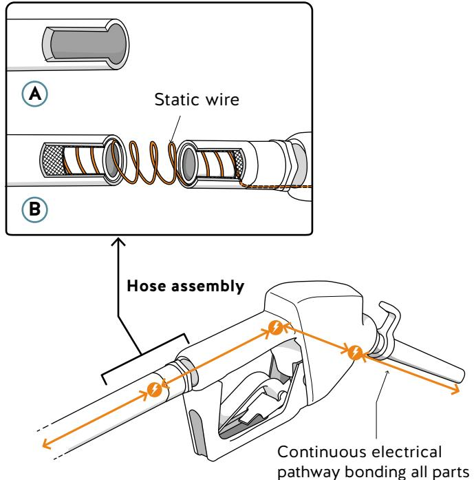
Cutaway views of a non-bonded fuel hose (A) and a bonded, ULC-approved fuel hose (B) next to a fuel nozzle. To reduce the risk of a static spark, the electrically bonded hose and nozzle must create a continuous path for electricity through all parts of the dispensing system. Note that nozzle designs may vary across industries.
