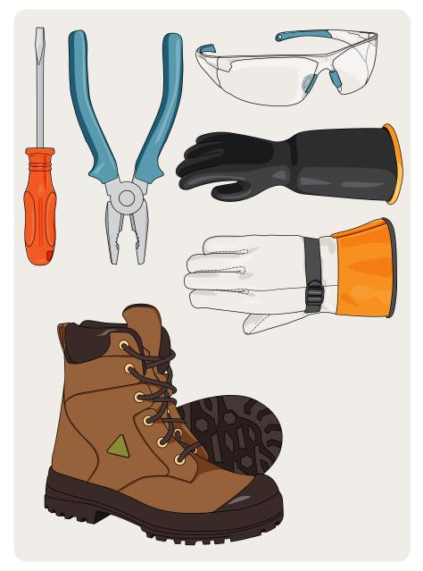
When working on energized low-voltage equipment, workers need protective equipment, including insulated tools, safety eyewear, rubber gloves, and shock-resistant footwear.
