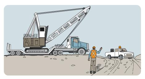
The boom of the grapple yarder has been lowered for transport under power lines.
