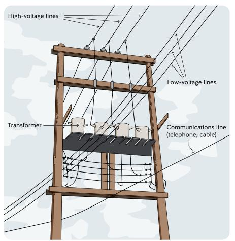
On older systems, transformer bank platforms may be installed using an H-frame configuration. They are most often seen in alleys. The illustration on page 3 shows a common single-pole configuration.
