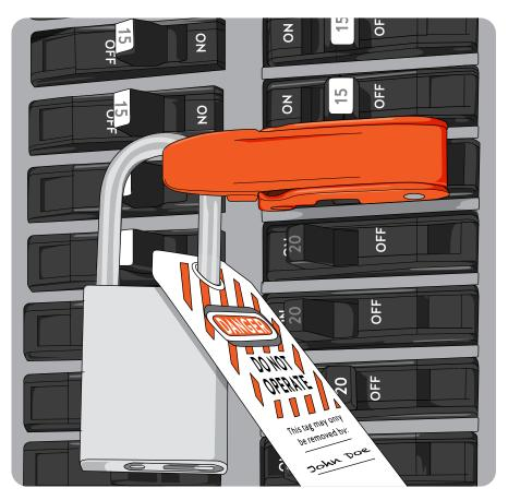
Lockout is required at the electrical panel before replacing any part associated with the lighting circuit.
