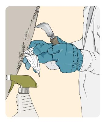
Use sampling tools to collect the desired sample. Place the collected sample in a sample bag.
