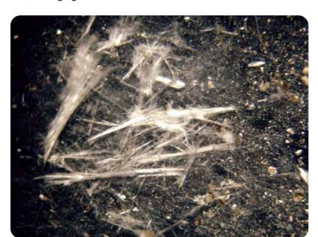
Asbestos fibres magnified many times
