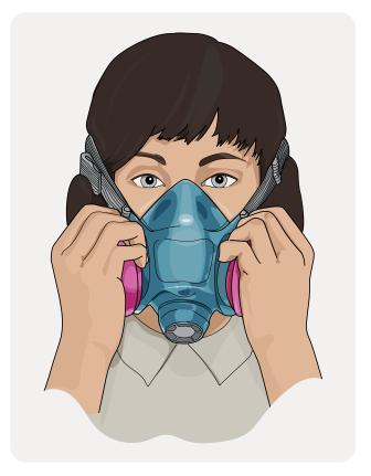
For a negative-pressure seal check, close off the inlet openings with your palms and inhale gently.
