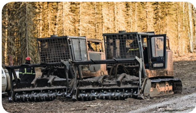
Mulchers with protective structures clear underbrush on the ROW.
