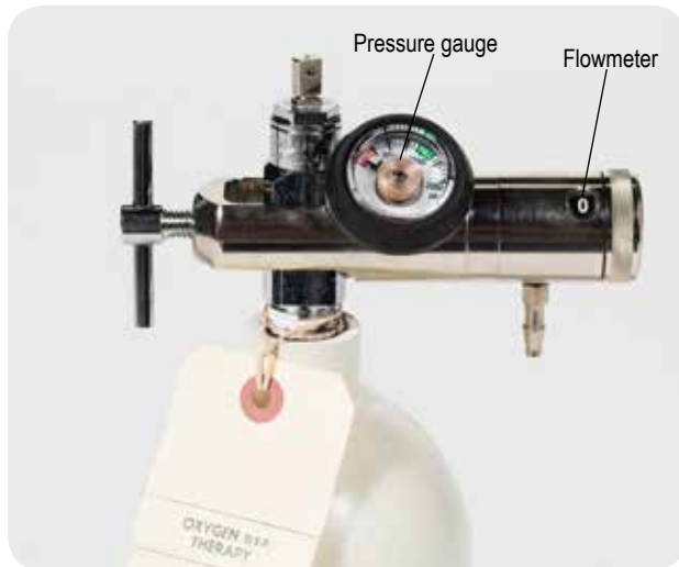
Figure - App D 4 Medical post-type cylinder showing pressure gauge and flowmeter
