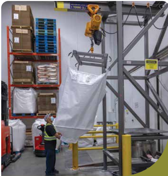
Jose Benitez, warehouse worker at Island City Bakery, operates an automated pulley system to swap out an empty bag of flour on this sifting machine.
