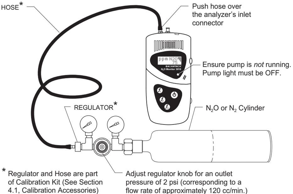
Figure 2. Applying Gas using Bacharach's Calibration Kit
