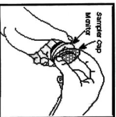
2. While holding Sampler with holes looking through the Holder's "cat face" cut-out, slide Sampler down and in until the Sampler's front rim rests in the "chin" of the "cat face". (Fig. 3)
