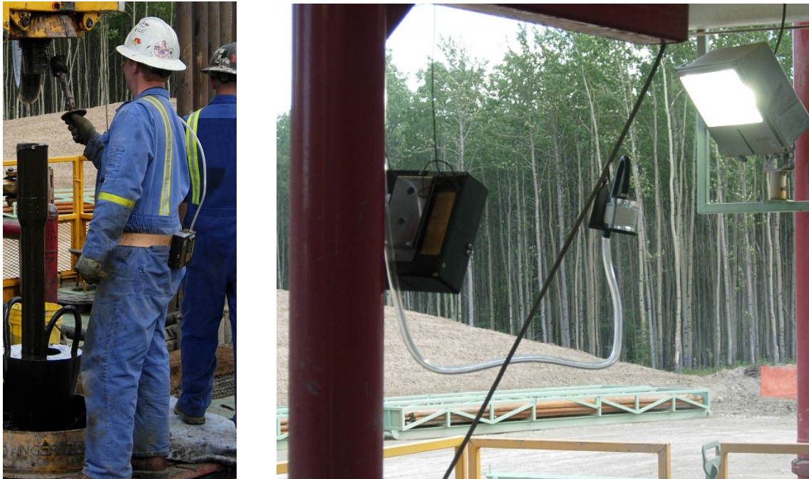
Figure 2: Typical Sampling setups (pump and cassette) on the Drill Rig (left – occupational sample on a Roughneck; right – area sample over Shakers)
