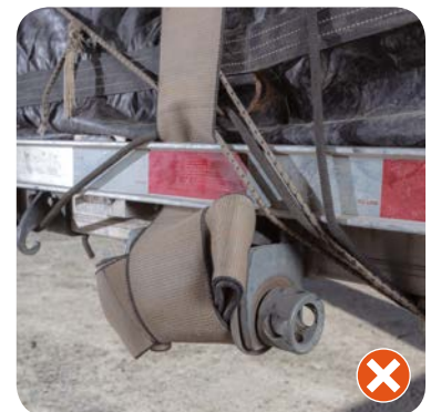
An improperly secured strap
