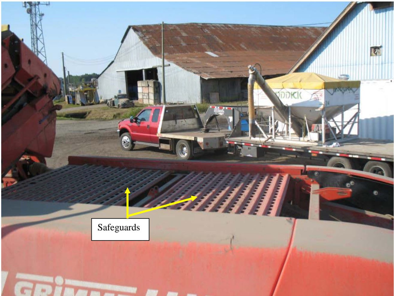
Figure 6: This photograph shows the safeguards that should have been installed over the haulm rollers. The safeguards are designed to keep workers from being pulled into the machine.
