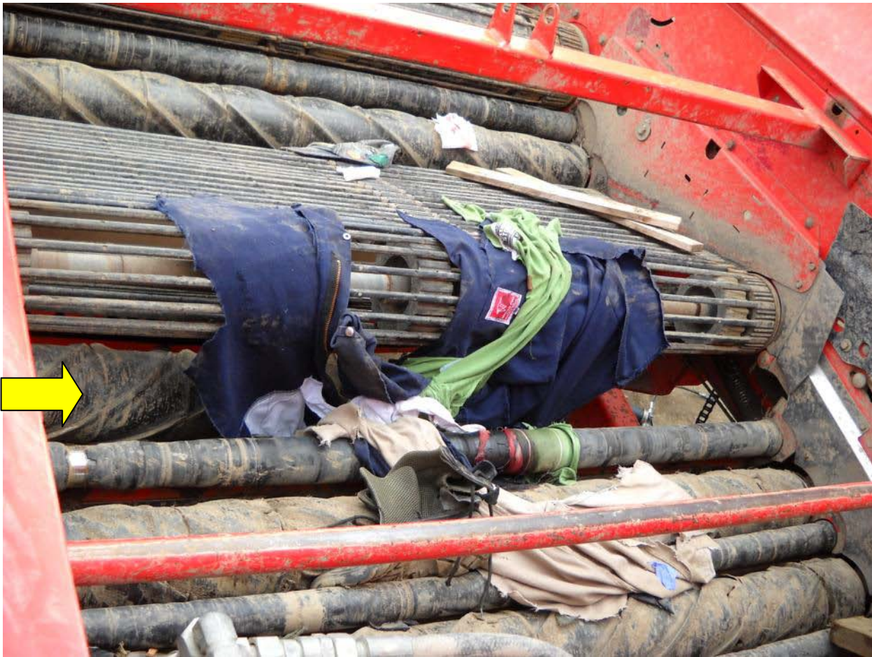
Figure 3: A view of where Worker 1 was trapped in the haulm rollers. The arrow identifies one of the haulm rollers.
