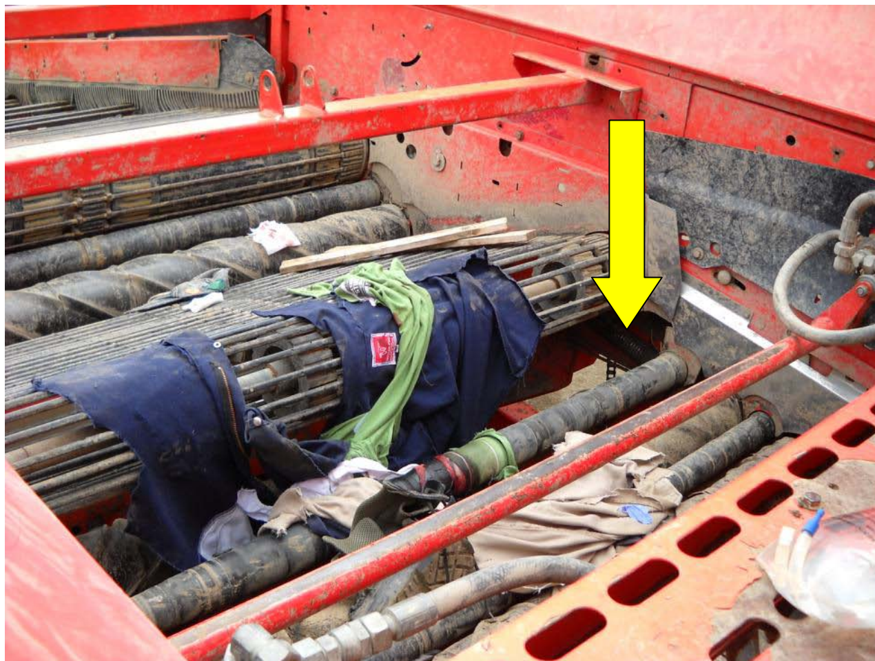
Figure 5: The arrow shows where Worker 1 was trapped in the unguarded haulm rollers.
