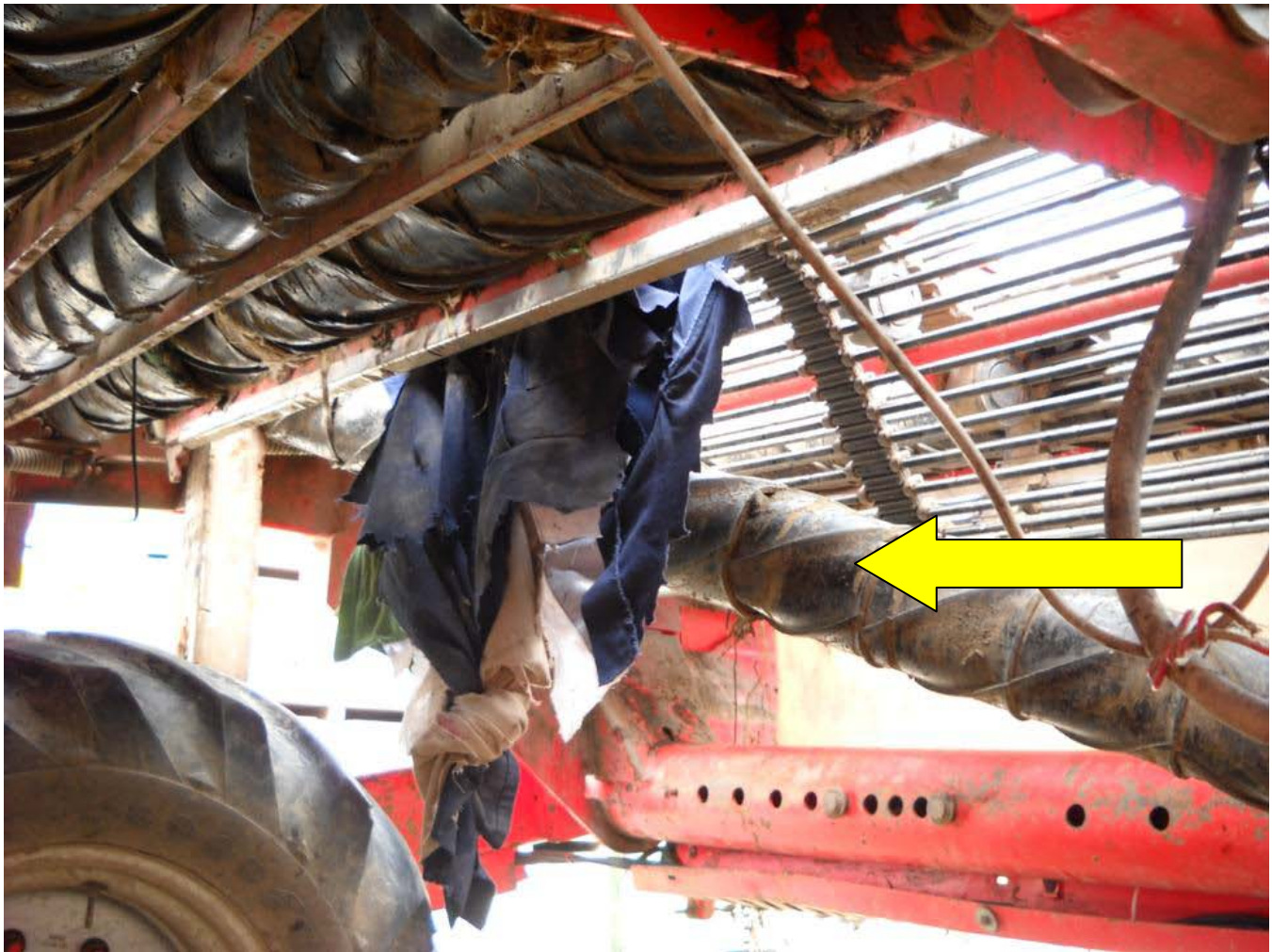
Figure 4: The arrow shows the haulm roller that pulled Worker 1's leg into the harvester and trapped it. Emergency responders had to drop the roller from its original position to extricate the worker.
