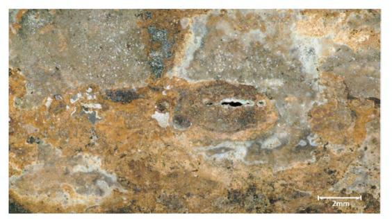
*Figure 26:* Close-up of the exterior of tube R2T3, showing the hole that allowed ammonia to enter the brine circulation system. (Source: Forensic Engineering Report from Acuren Group Inc. — Appendix C)
