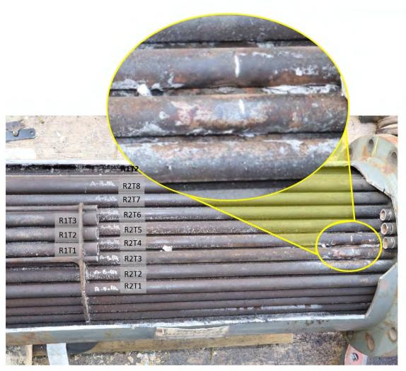
*Figure 24:* Photograph with close-up showing radial patterns and corrosion in the second row of brine tubes at the outlet end of the curling rink chiller.
