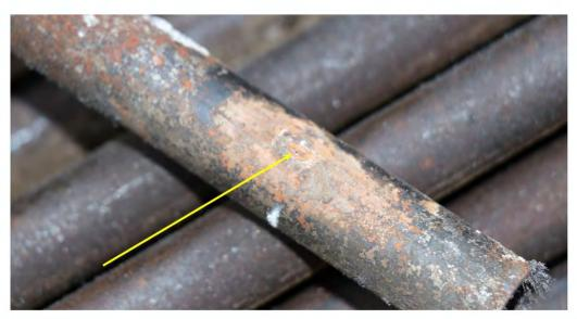
*Figure 25: Photograph showing brine tube R2T3 after removal from the tube bundle. WorkSafeBC investigators observed a small hole in the tube (yellow arrow).*
