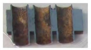
*Figure 23: Three brine tubes cross-sectioned at the tube plate. Examination showed good mechanical connection of the rolled tubes with no evidence of leaking.*
