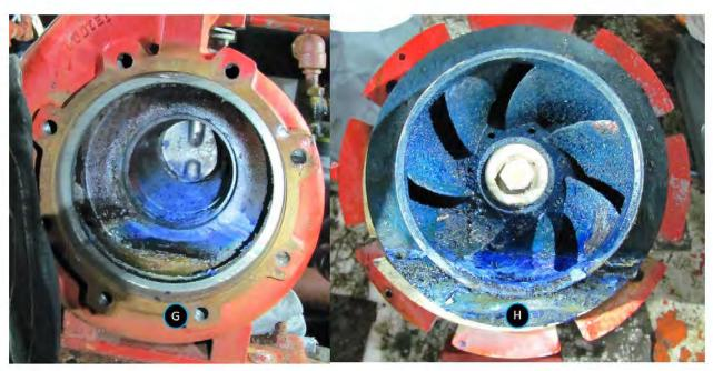
*Figure 12:* The interior of the curling rink brine pump housing (G) and the pump impeller (H), showing the corrosive effect of ammonia to some metals in the system, in this case the copper alloy/bronze pump impeller.
