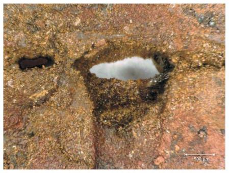
**Figure 27:** Close-up of the hole from the inside of brine tube R2T3. Scouring from the flow/jetting of material into the brine tube can be seen directly below the hole. Other pits have developed on both sides of the breach. (Source: Forensic Engineering Report from Acuren Group Inc. — Appendix C)
