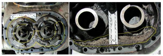
*Figure 15:* Crystal accumulation (yellow outline) in the ammonia gas compressor cylinder heads, showing cylinder heads on the left and a cylinder head cover and springs on the right.
