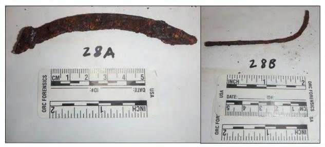
*Figure 21:* Two metal pieces found at the inlet end of the curling rink brine tube sheet. (Source: Forensic Engineering Report from Acuren Group Inc. — Appendix C)
