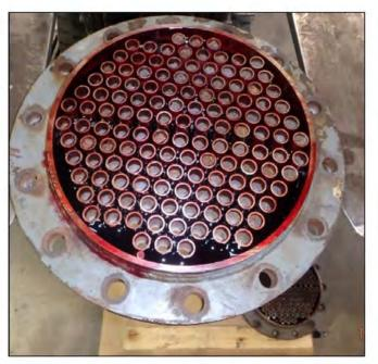
**Figure 22:** The cross-sectioned tube sheet in the foreground; the second sheet is in the lower right corner of this photograph, with the ammonia pressure shell end facing up. A red penetrating dye bath has been added to test for permeation through the tube sheet. (Source: Forensic Engineering Report from Acuren Group Inc. — Appendix C)
