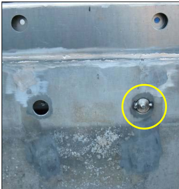
Figure 2: Close-up view of the exterior of the transom. The first bung (circled) has been inserted and tack-welded into one of the four new bolt-holes.
