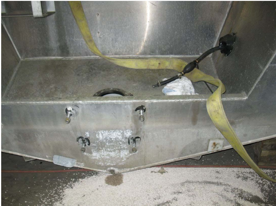
Figure 7: This photograph of an identical but undamaged vessel shows the sending line (black hose with a fuel priming bulb) entering the engine well through the hole from the battery compartment.
