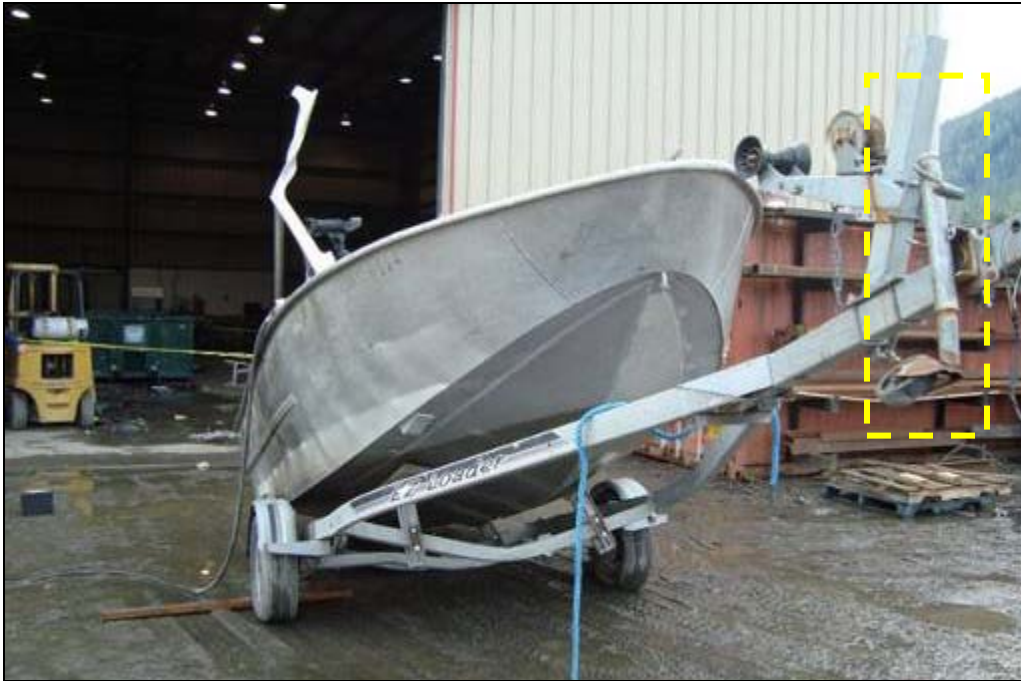
Figure 4: The boat and trailer parked outside the shop after workers wheeled the trailer through the overhead bay door. The damaged trailer jack and the bent small wheel components on the reach of the trailer are seen within the dashed rectangle.
