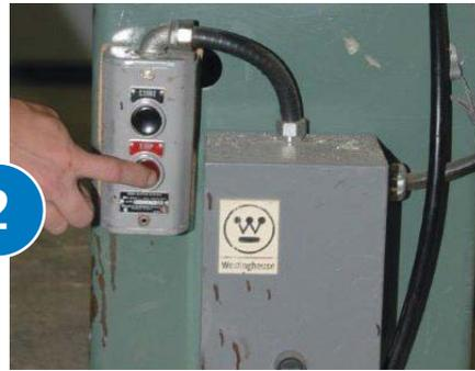
Turn the machine off and ensure that all moving parts have stopped.
