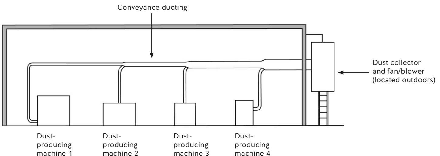
This diagram gives an overview of a typical dust collection system at a manufacturing facility.
