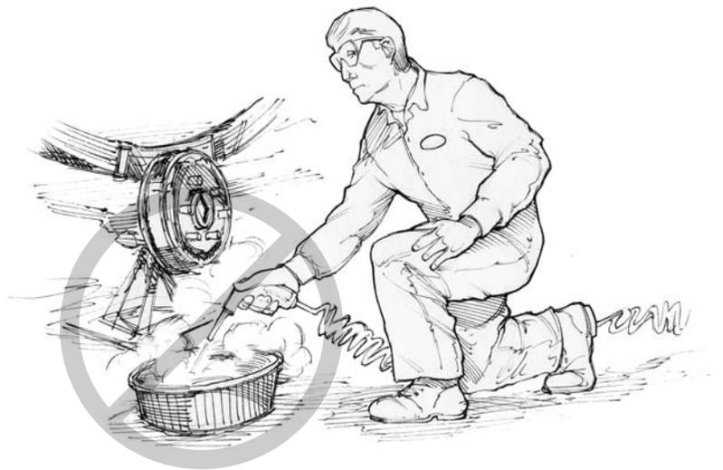
*Never use compressed air to remove dust from automotive friction materials. Even if the worker here was wearing a respirator, others would still be exposed to airborne asbestos dust.*
