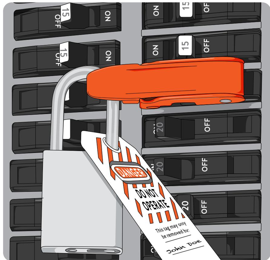
Lockout is required at the electrical panel before replacing any part associated with the lighting circuit.
