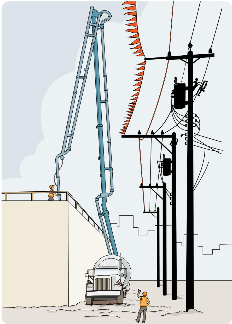
Guarding is a visual warning only. The grounded guard wire (with flags) gives warning of approach. The overhead line cover-up, installed by the owner of the power system, has no insulated rating for the purposes of Form 30M33. Workers and equipment must not contact the guard wire or overhead line under any circumstances.
