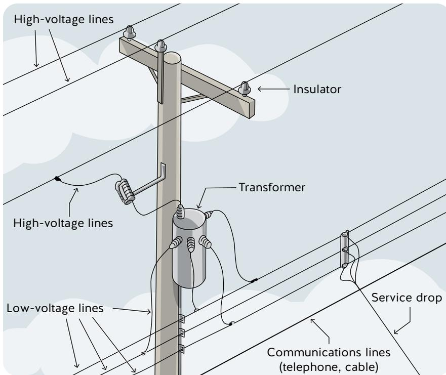
You can often identify overhead electrical conductors by their placement on the pole.
