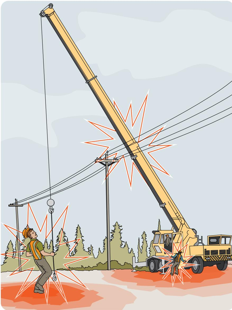
If mobile equipment touches a power line, electricity can travel from the power line to a worker touching any part of the equipment, including a pendant control.
