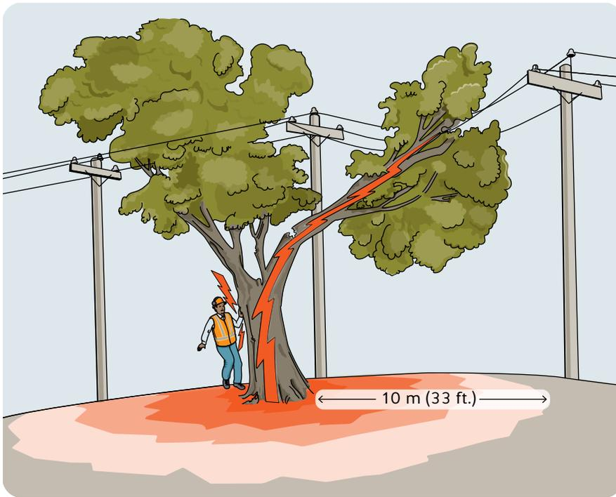
If anything, such as a tree or equipment, touches a high-voltage power line or if a power line falls to the ground, electricity will flow to the ground. This will energize the tree or equipment and anything in contact with it. The surrounding ground may be extremely hazardous. The voltage gradually decreases from the point of contact until it reaches zero.
