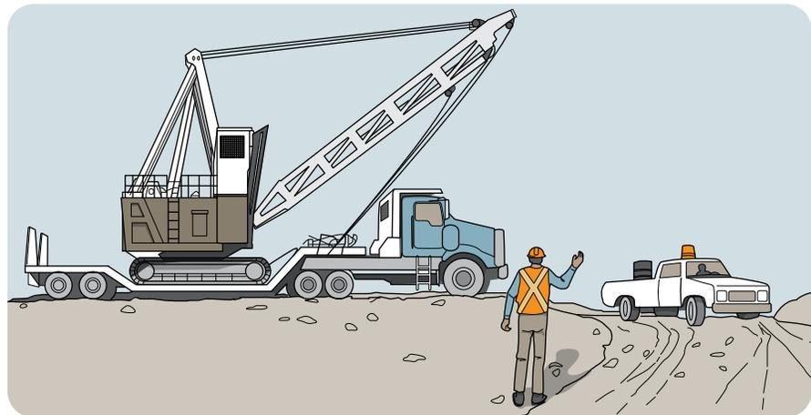
The boom of the grapple yarder has been lowered for transport under power lines.
