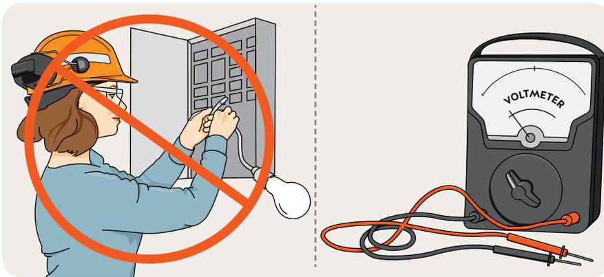
Use approved portable meters and leads, not improvised test lamps.
