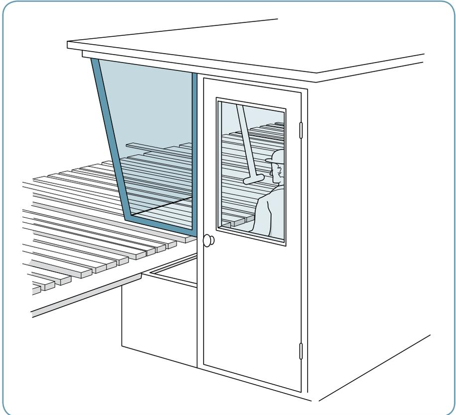
A partial operator booth helps reduce noise levels while allowing the operator to handle material.
