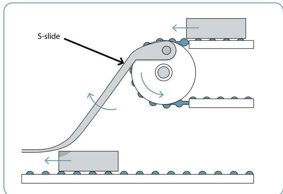
An S-slide will reduce drop height and deliver material quietly.
