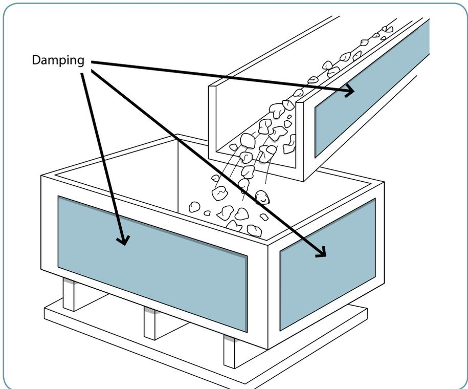
Installing damping in delivery chutes and bins will reduce noise.
