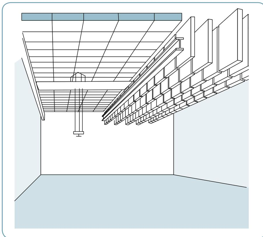
Sound-absorbing baffles help reduce reflected noise.
