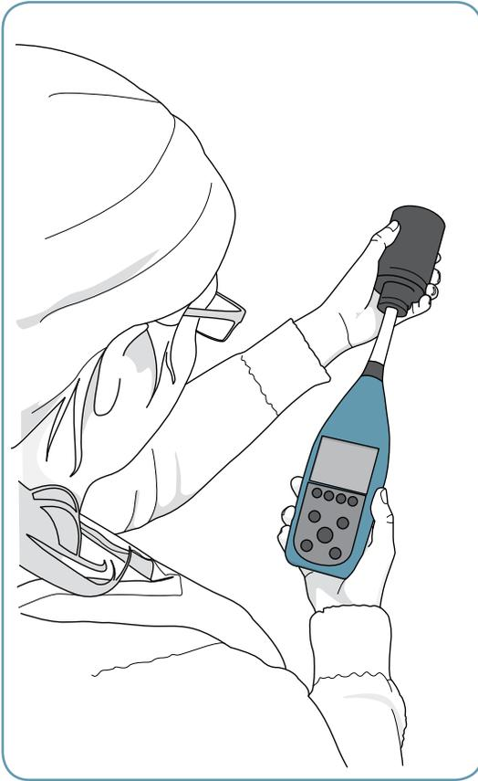
Integrating sound level meters average noise levels over time. To ensure proper function, these should be calibrated before and after a survey.
