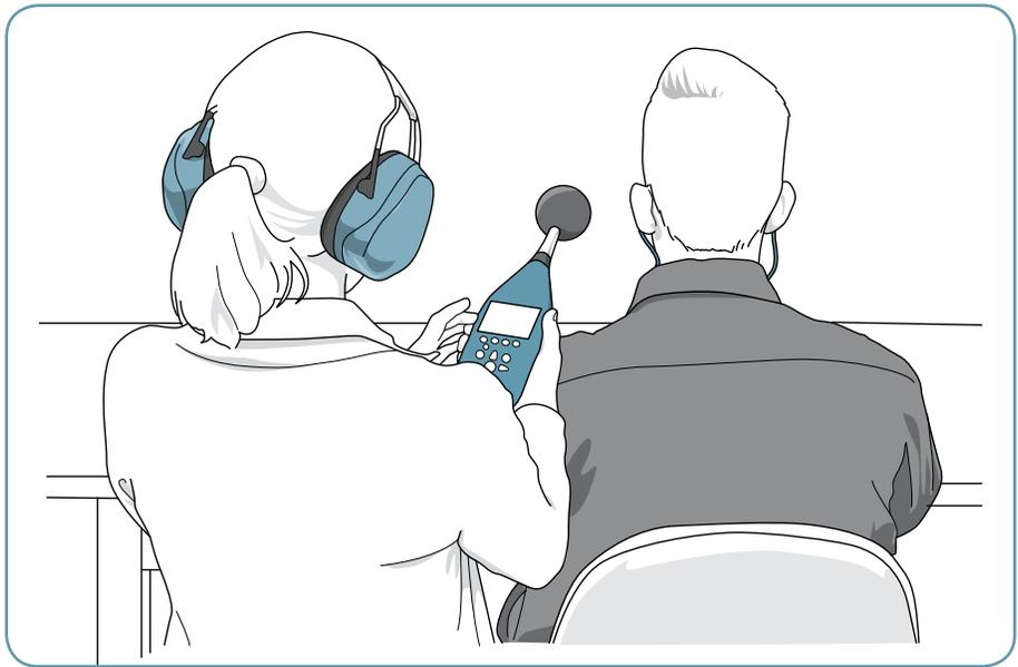
When measuring noise levels (for example, with a sound level meter, as shown in the illustration), position the microphone in the worker's hearing zone on the side where there's the most noise.
