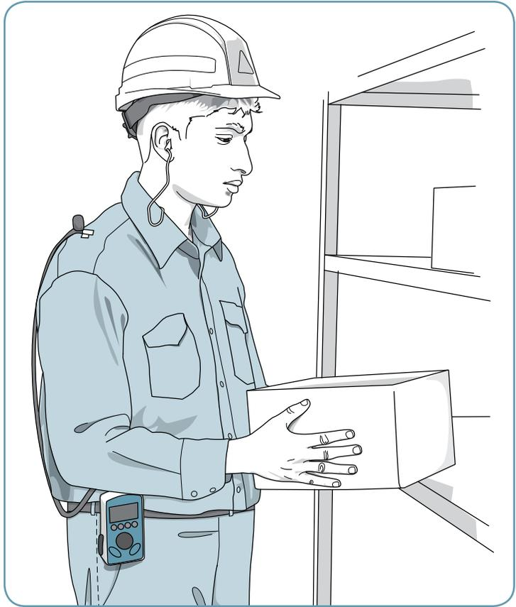
Workers wear noise dosimeters over the shoulder or on the collar.
