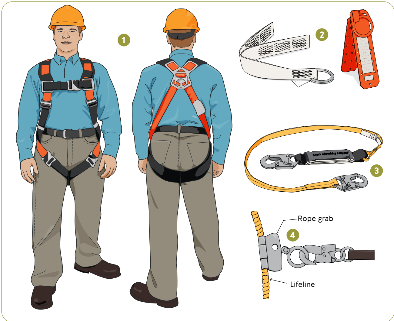
1. Personal fall protection harness. 2. A synthetic webbed anchor strap and a metal roof anchor (ridge anchor). 3. A shock-absorbing lanyard. 4. A vertical lifeline with an attached rope grab and lanyard.
