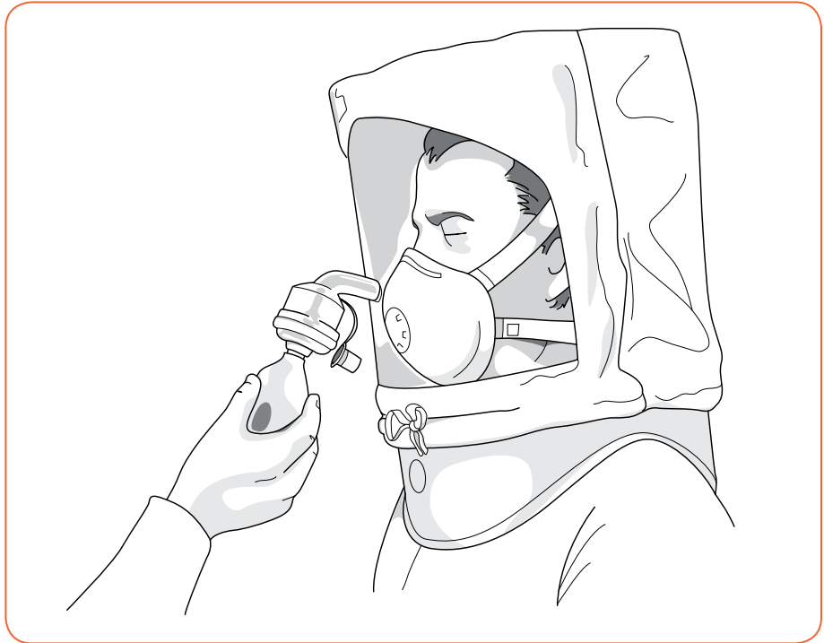
Fit testing for a single-use respirator using a special hood
