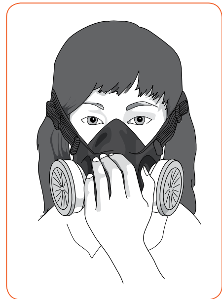
Positive-pressure seal check
