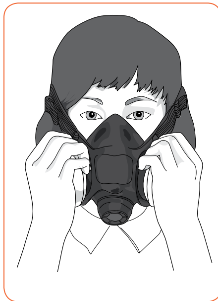
Negative-pressure seal check for a half-facepiece elastomeric respirator
