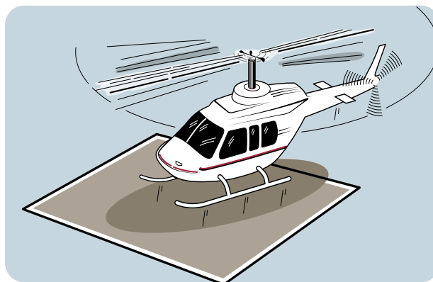
Figure 50-5 Keep the landing site free from loose debris
