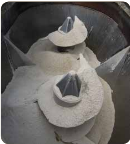
Mechanical equipment in a feed mixer
