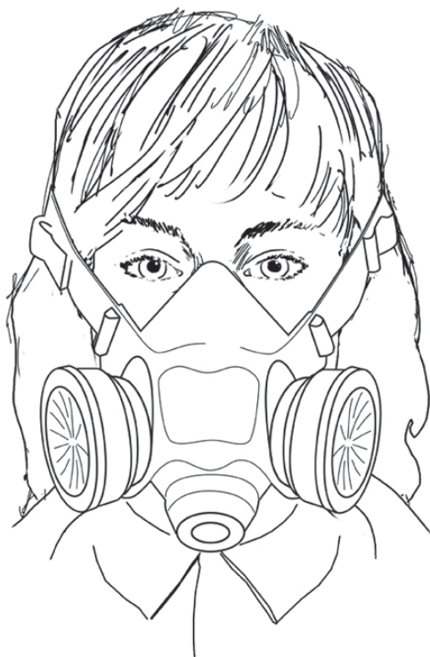
Half-facepiece respirator with cartridges.
