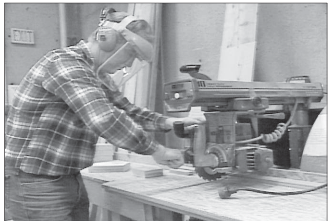
Keep the plug in plain view and within reach while changing the blade.
