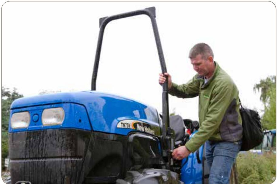
A familiar example of an engineering control for a long-standing hazard is the use of a rollover protective structure (ROPS). Control measures that are built in by design are reliable and their success does not depend on individual judgment, training, or decision-making.
