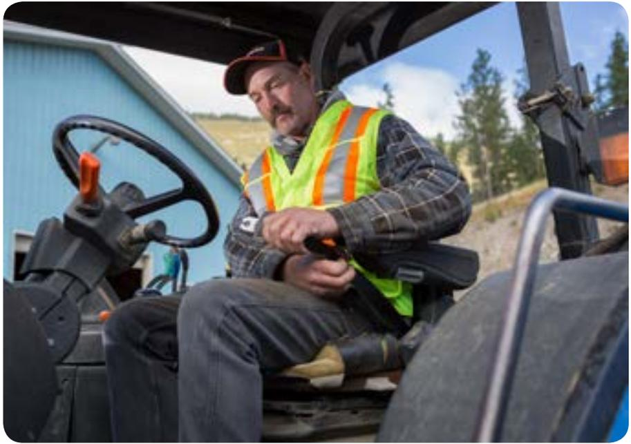
If a machine is equipped with a rollover protective structure, make sure your seat belt is securely fastened.
