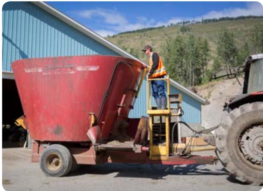
Feed mixers must be fitted with adequate safeguards that prevent access to hazardous points of operation.
