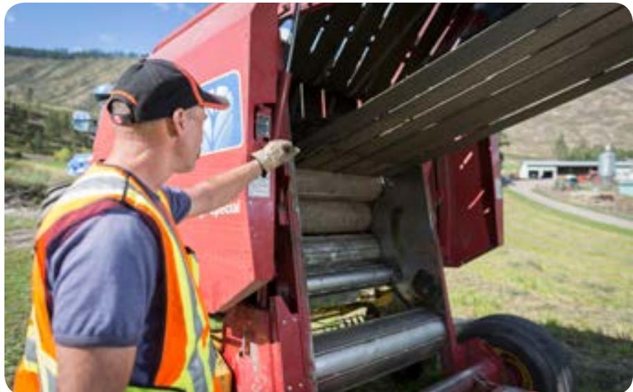
Always de-energize and lock out equipment before doing any cleanup, maintenance, or repairs.
