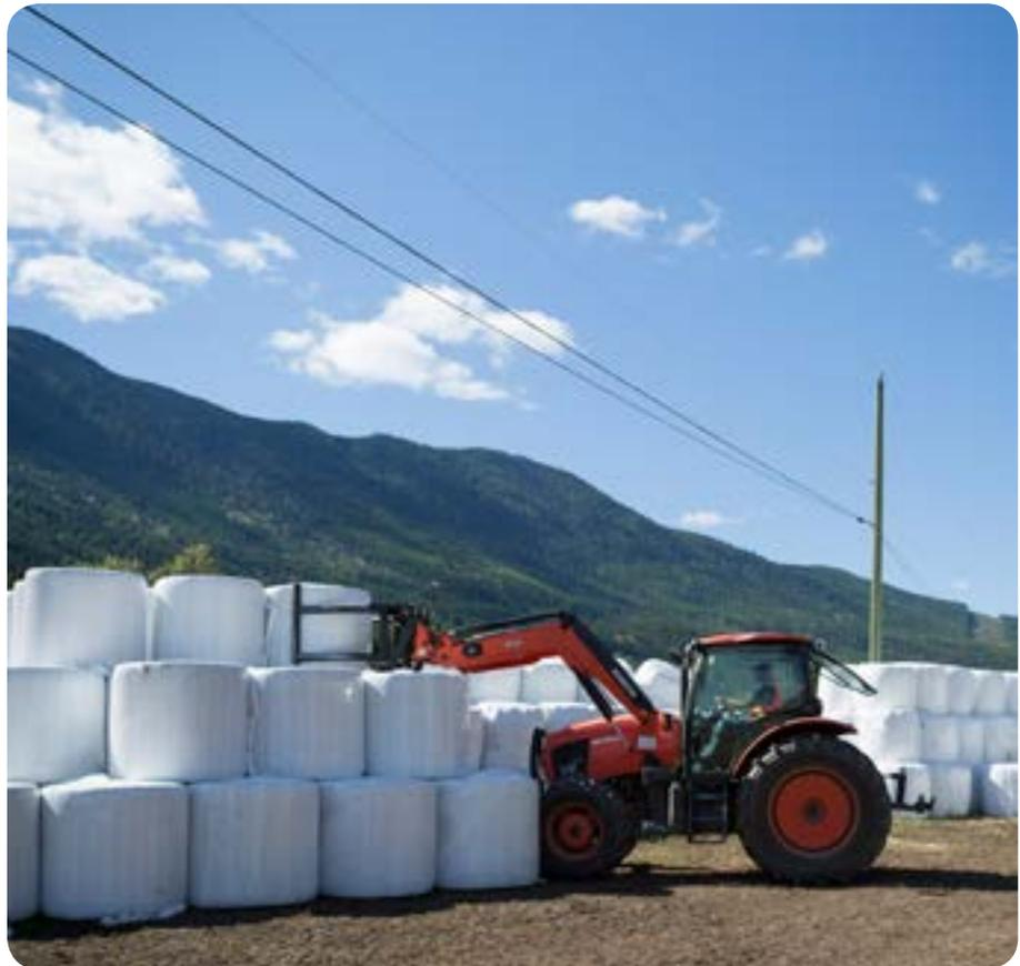
When operating mobile equipment near power lines or electrical equipment, maintain the limits of approach specified in Part 19 of the Regulation.
