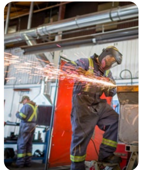
Tycorp employee grinding welds on finished product.
