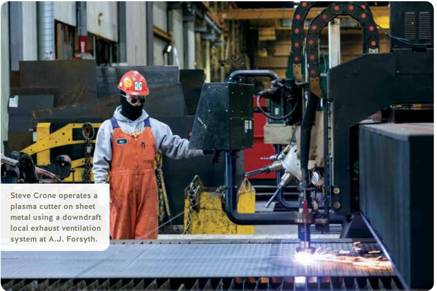
Steve Crone operates a plasma cutter on sheet metal using a down-draft local exhaust ventilation system at A.J. Forsyth.
