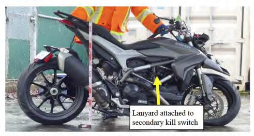
Figure 3: The motorcycle, showing the location of the secondary kill switch.
