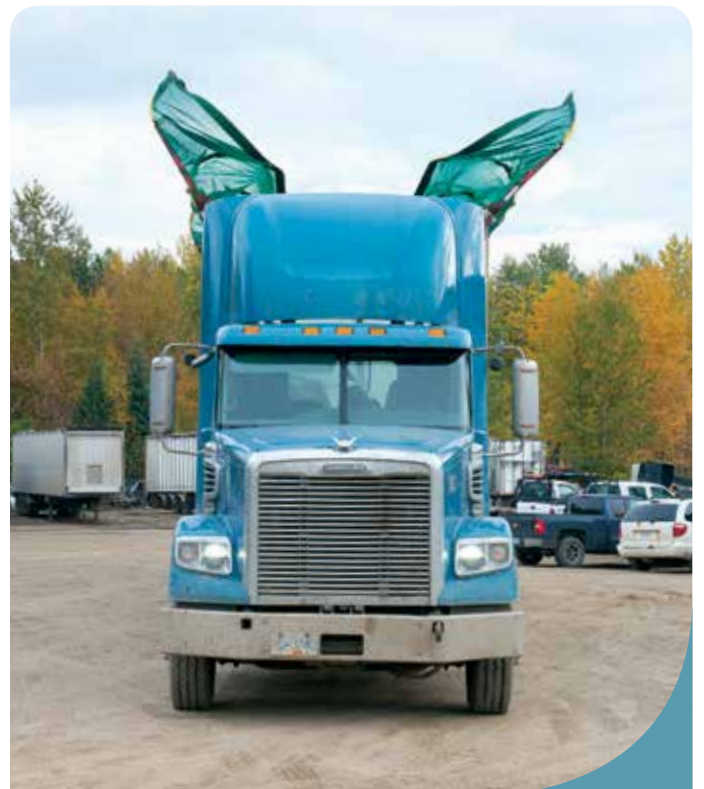
In this truck, the tarps are operated from inside the cab, as demonstrated by shop foreman Dave Kerr.
