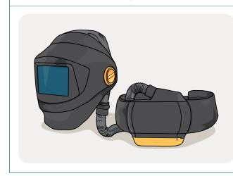
PAPRs are available with an integrated welding visor to protect the skin and eyes from UV and to provide a clear viewing window. This device allows a welder to keep the respirator in place when checking a weld. If a welder has to lift the visor to check a weld, they should wait until visible fumes have disappeared before doing so.
