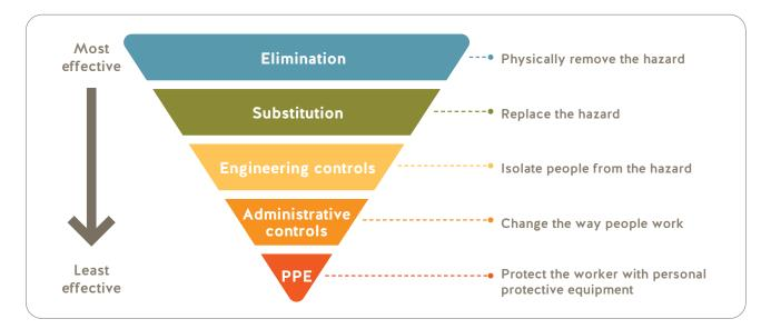
Even though the controls are listed in order of effectiveness, you should consider all types of controls. They often work best in combination — for example, using a respirator in addition to LEV.
