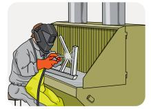
Extracted workbenches are ideal for workpieces that can be transported to the workshop.
