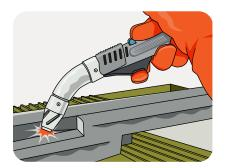
On-torch capturing hoods are useful when welding larger workpieces that are too big to transport to a workbench.
