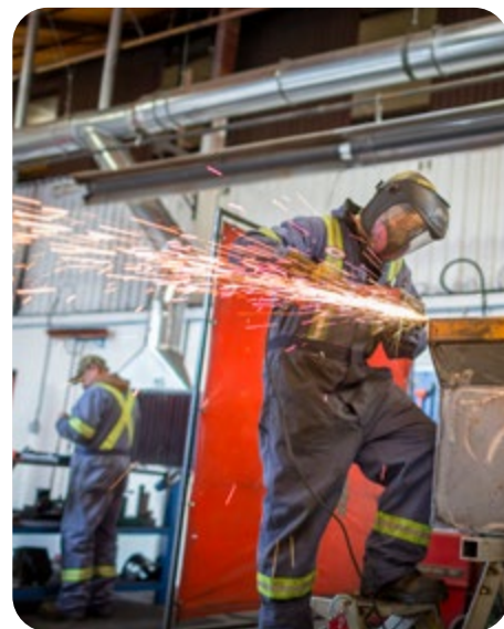
Tycorp employee grinding welds on finished product.
