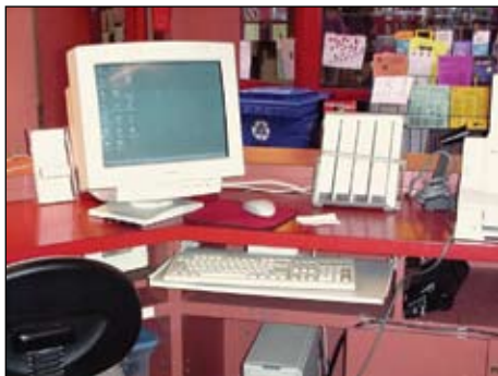
Incorrect monitor position
