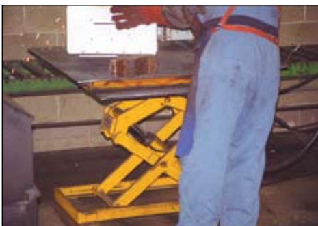
Working at an appropriate level by using a scissor lift
