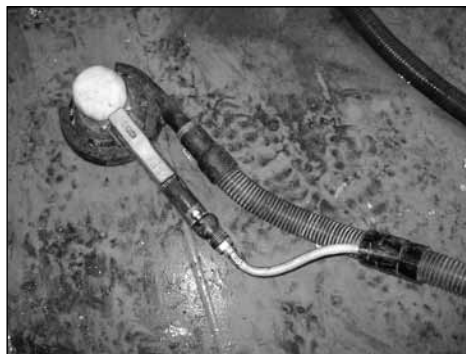
Grinder with a HEPA exhaust attachment
