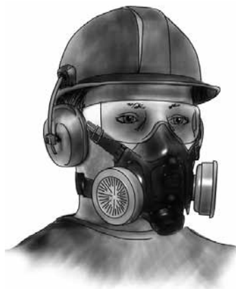
Half-facepiece elastomeric respirator with HEPA cartridges
