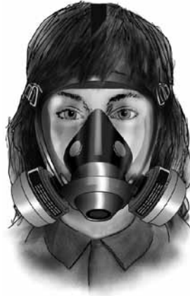
Full-facepiece elastomeric respirator with HEPA cartridges
