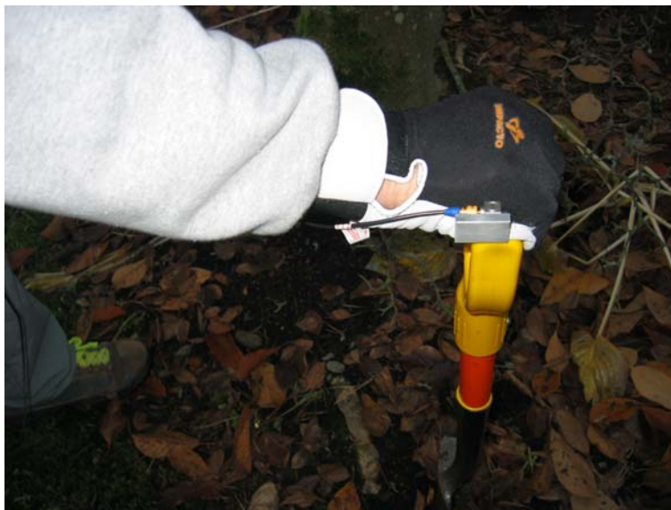
Figure 8. Tree planting shovel with Impacto anti-vibration glove and bar type accelerometer adaptor inserted between the glove and the palm of the hand.
