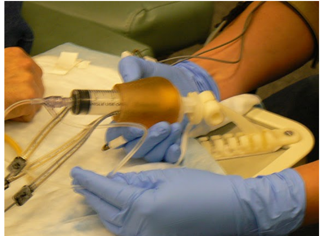
Figure 2. Force sensors on standard syringe Figure 3. Force sensors on adapter
