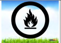
This symbol means flammable. If you see this on any chemicals, substances, or equipment, be sure not to expose it to open flames or high heat. In particular, this would not be a good place for a cigarette break!
