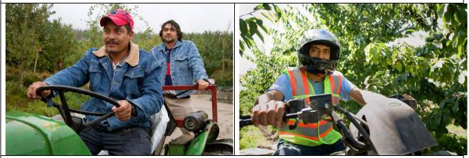
This first image is a hazard because of the worker riding on the back of the tractor, which is unsafe. The second image shows a worker wearing a helmet and a visibility vest, which is good safety practice.
