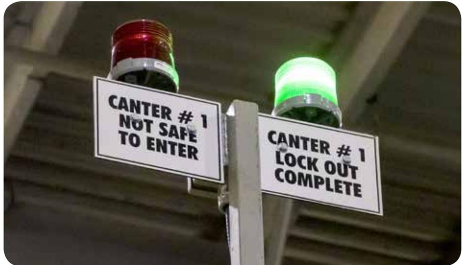
Figure 6: An indicator showing that it is safe to enter the area.
